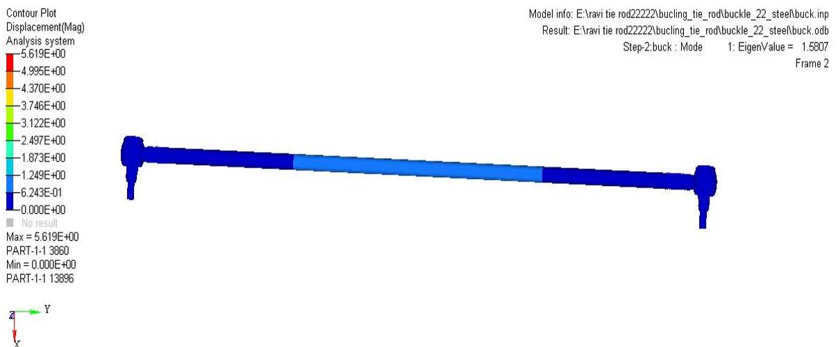
Fig.4: Buckling eigen value at 1.5807
