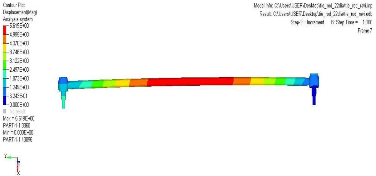
Fig.2: Displacement at 5.619mm
